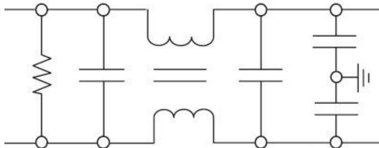
Fig 2: EMI Filter Schematic
