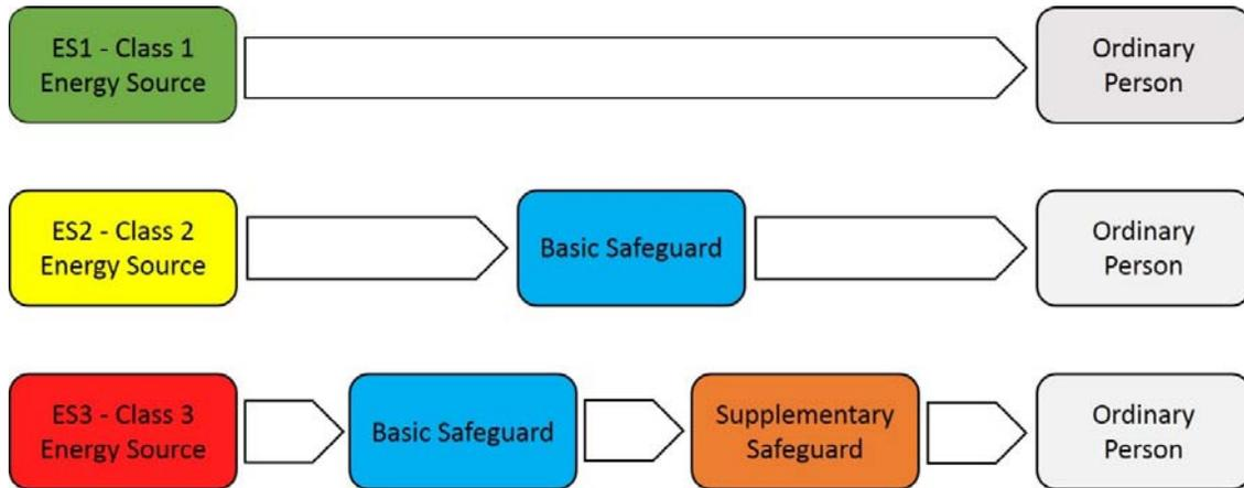
Figure 1: Protection for an Ordinary Person with different Energy Classes
