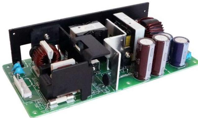
Although based on TDK-Lambda's ZWS300BAF-24 which is OVC II, it has increased spacing from the Line and Neutral to ground, including additional spacing on the input connector. It is also certified to EN 62477-1 - safety requirements for power electronic converter systems and equipment. It is said to be a more suitable specification than EN 50178 which covers electronic equipment for use in power installations.
