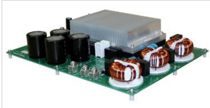
In all situations, the system must be tested with the selected fan and all other devices in-place to confirm that the power supply or converter and the load it drives do not exceed their maximum operating temperature, under worst case conditions (maximum ambient inlet air temperature, 100% power load, etc.). If problems are observed, a higher CFM rated fan or dual fans may be required.
