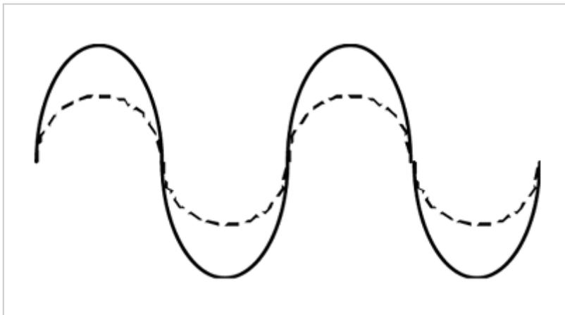
**Figure 2. Voltage and Current waveforms are sinusoidal and in-phase; PF=1.**
