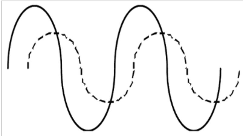
**Figure 1. Voltage and current waveforms are sinusoidal but out-of-phase; PF < 1.**
