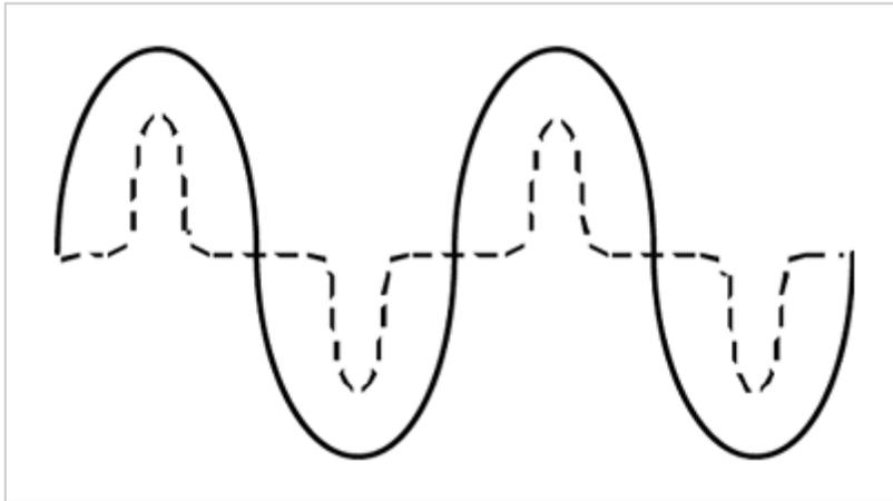
**Figure 3. Voltage waveform is sinusoidal, current waveform is non-sinusoidal but in-phase; PF<1.**
