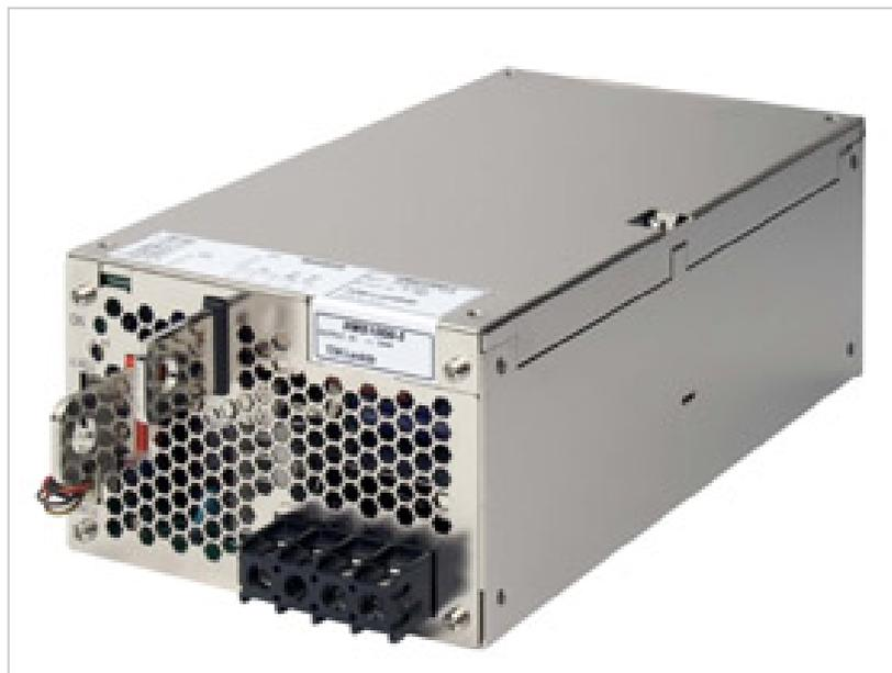
Photo #2: This 1000-watt switch-mode power supply is 3.25" high and, therefore, can be mounted in a 2U rack-mountable enclosure, which can vary between 3.44" to 3.50" high.
