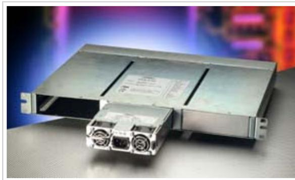
Photo #1: This 19" rack-mountable power system can hold up to 3 plug-in, hot-swap and redundant power supplies. The enclosure with mounting ears is 1.72" high (= 1.75" minus 0.03") and is therefore considered 1U high.
