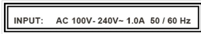
However, a close look at the power supply's datasheet will usually show the absolute AC input voltage range, from minimum to maximum. This is usually 90-264VAC, or occasionally 85-264VAC if the power supply has been designed for Japanese use.
