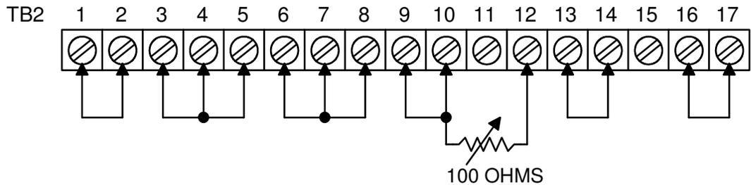
FIGURE 4: REMOTE PROGRAMMING BY EXTERNAL RESISTANCE, CURRENT MODE
