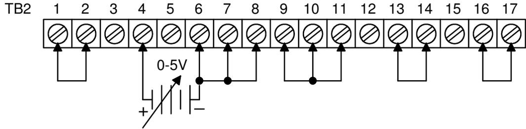
FIGURE 5: REMOTE PROGRAMMING BY EXTERNAL VOLTAGE, VOLTAGE MODE
