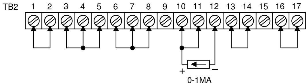
FIGURE 8: REMOTE PROGRAMMING BY EXTERNAL CURRENT, CURRENT MODE
