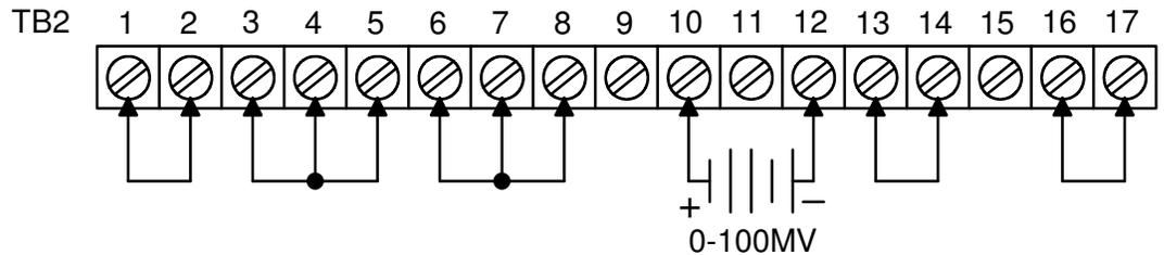
FIGURE 6: REMOTE PROGRAMMING BY EXTERNAL VOLTAGE, CURRENT MODE
