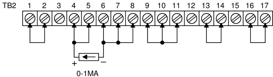
FIGURE 7: REMOTE PROGRAMMING BY EXTERNAL CURRENT, VOLTAGE MODE
