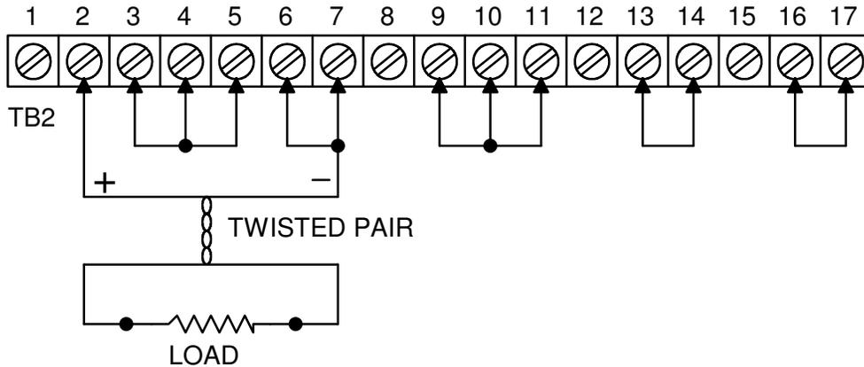
FIGURE 2: REMOTE SENSING
