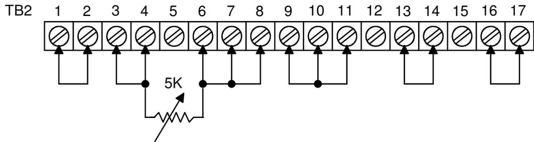
FIGURE 3: REMOTE PROGRAMMING BY EXTERNAL RESISTANCE, VOLTAGE MODE
