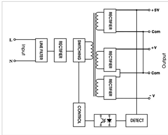
On the middle right hand side of the diagram are the three output windings from the transformer.
